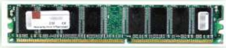
Picture of a RAM; a one giga RAM can keep information equivalent to one million words
